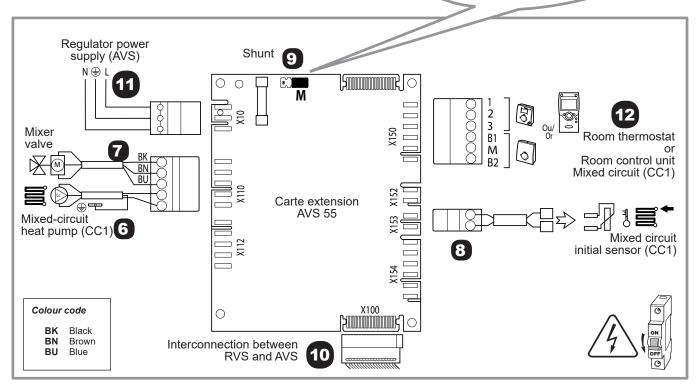
figure 13 - Electrical connection on AVS 55 extension board
