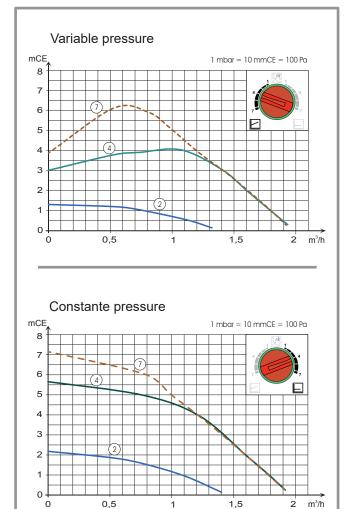
figure 2 - Hydraulic pressures and flow rates available (Hydraulic unit + 2nd circuit kit)
