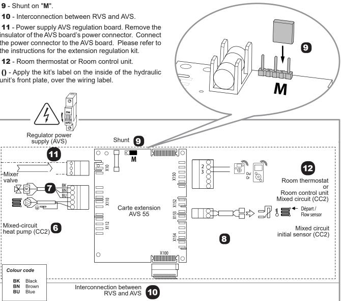
figure 5 - Electrical connection on AVS 55 extension board
