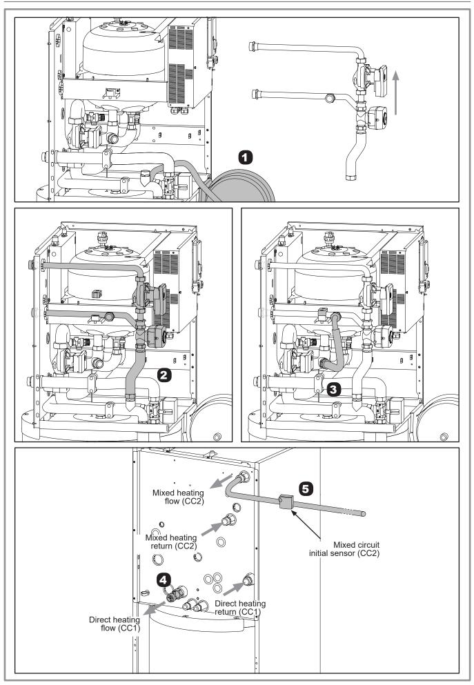
figure 4 - Installing the hydraulic kit
