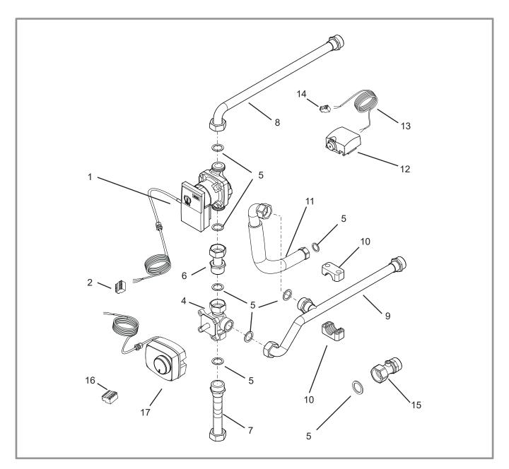
figure 14 - Spare parts 2nd circuit kit
