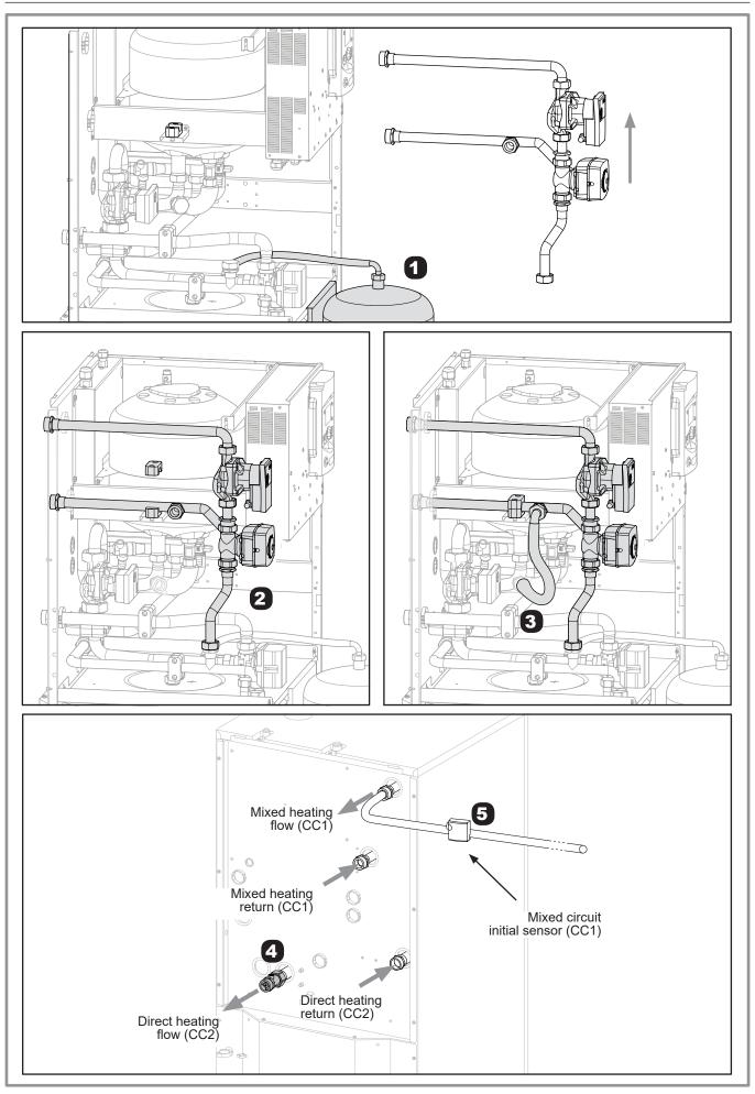
figure 11 - Installing the hydraulic kit
