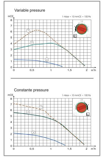
figure 8 - Hydraulic pressures and flow rates available (Hydraulic unit + 2nd circuit kit)
