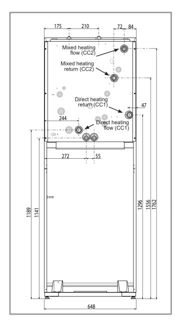
figure 1 - Dimensions in mm
