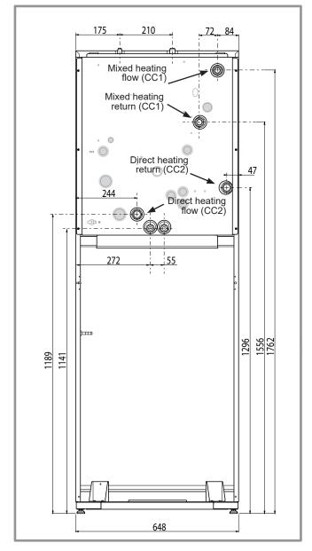
figure 9 - Dimensions in mm
