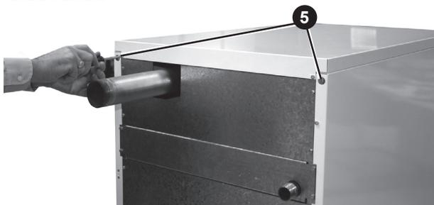
6. Undo the 2 screws at the rear and the 2 screws at the front of each panel.
