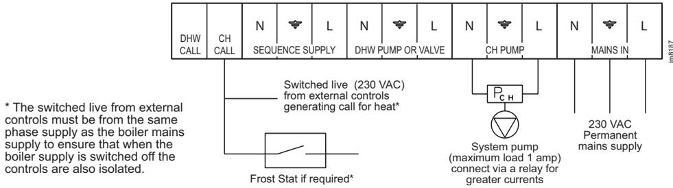
\* The switched live from external controls must be from the same phase supply as the boiler mains supply to ensure that when the boiler supply is switched off the controls are also isolated.
