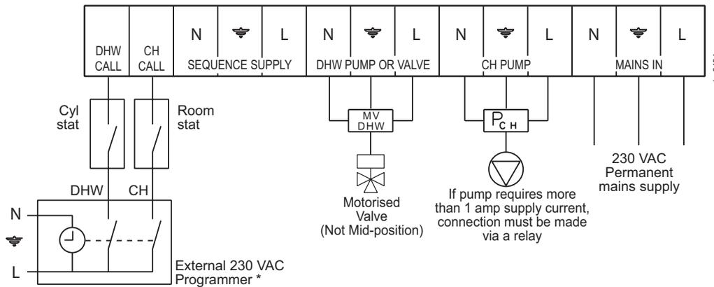
\* The switched live from external controls must be from the same phase supply as the boiler mains supply to ensure that when the boiler supply is switched off the controls are also isolated.
